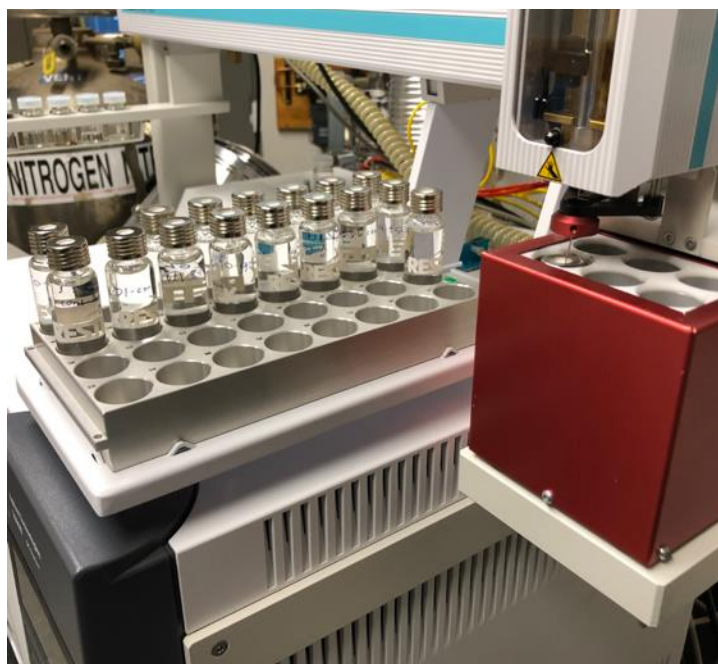
Figure 5.2.1.1. Samples in the process of SPME analysis on the GCxGC/TOFMS.
