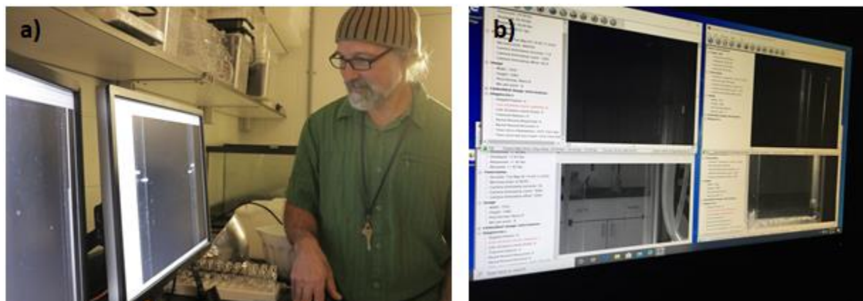
Figure 4.7.1.2. Monitors to inspect camera settings and live video feeds. a) Image depicts monitors linked to cameras outside of the experimental room with b) view of the computer monitor capturing images from 4 cameras simultaneously from four quadrants along the experimental chamber.
