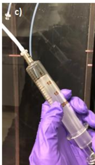
Figure 4.6.1 Chemical sampling system. a) Diagram shows the sampling port system throughout the experimental chamber. b) Image of individual sampling port situated near the surface of the experimental chamber. c) glass syringe used to extract water samples attached to the end of a teflon tube corresponding to the sampling port in image b.
