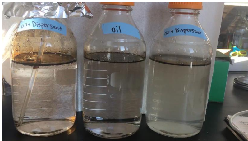
Figure 5.3.1.1. Prepared WAF and CEWAF water for small-scale experiments
